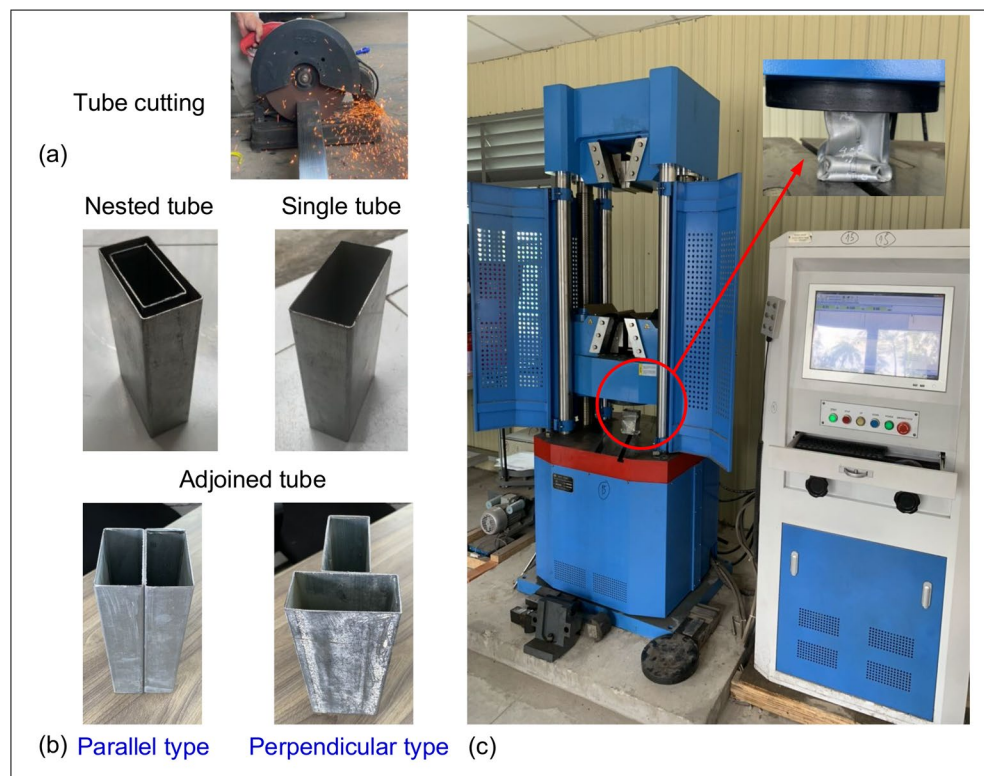
Fig. 2 (a) Tube cutting, (b) Tube arrangement and (c) Testing apparatus
