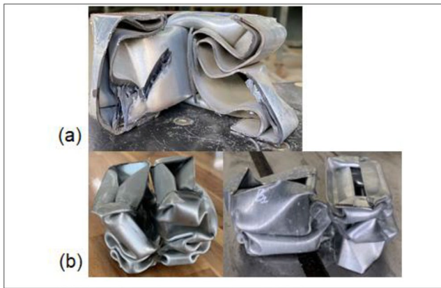
Fig. 12 Difference in deformation of constituent tubes: (a) Nested tube and (b) Adjoined tube
